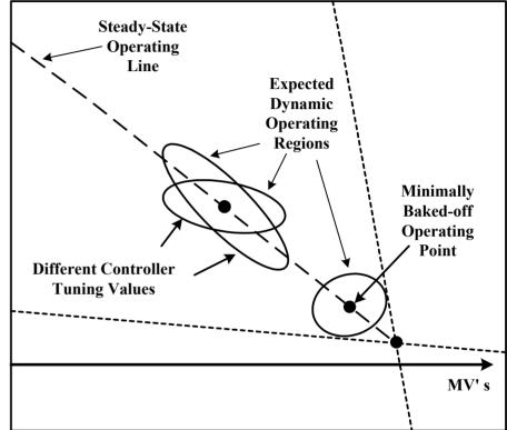
**Steady-State Operating Line:** Backed-off Points further limited by the Steady-State model.
